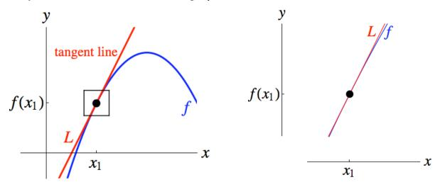
The **slope** of the tangent line is given by  $f'(x_1)$  or, more generically, by f'(x), so changes along the tangent line are related by the following formulas:
