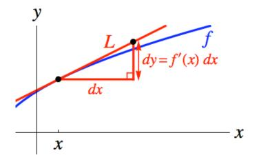
$\Delta x$  and  $\Delta y$  are the <u>increments</u> of x and y, respectively. They represent **actual changes** in x and y along the graph of f. • If x changes  $\Delta x$  units from, say,  $x_1$  ("**seed, old x**") to  $x_1 + \Delta x$  ("**new x**"), then y (or f) changes  $\Delta y$  units from  $f(x_1)$  to  $f(x_1) + \Delta y$ , or  $f(x_1 + \Delta x)$ .
